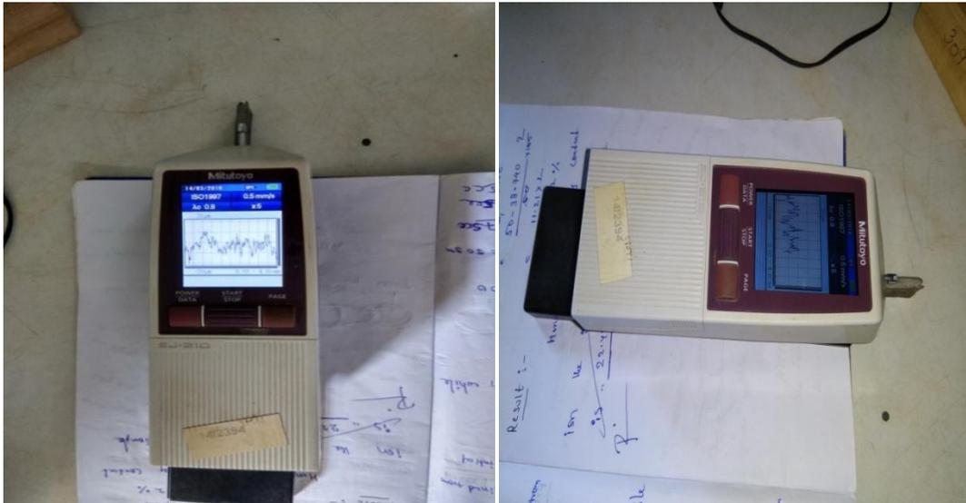
*Fig.6 & 7: Surface roughness tester*
